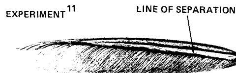
Fig. 11 Flow separation pattern on a prolate spheroid at \alpha = 30 deg and V_\infty = 147.6 ft/s.
